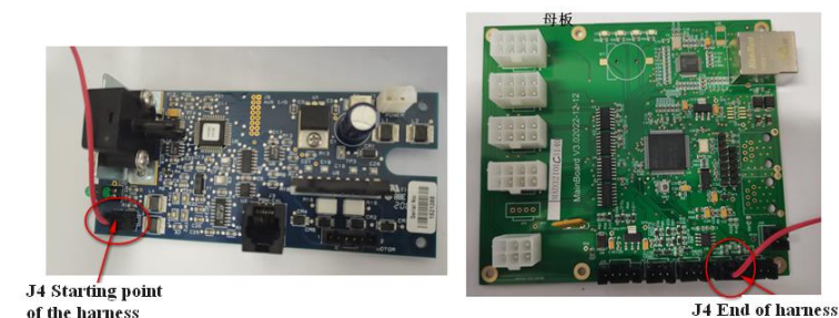
Figure 5-10 Connecting the deaerator J4 wiring harness
