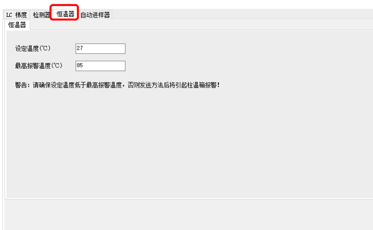
Figure 3-4 Temperature setting interface of the Kromstation workstation column oven
