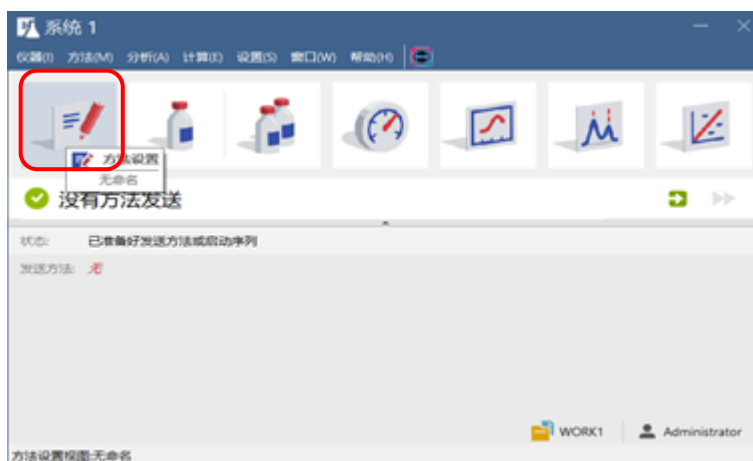
Figure 3-5 Instrument method setting interface of the W5100 workstation
