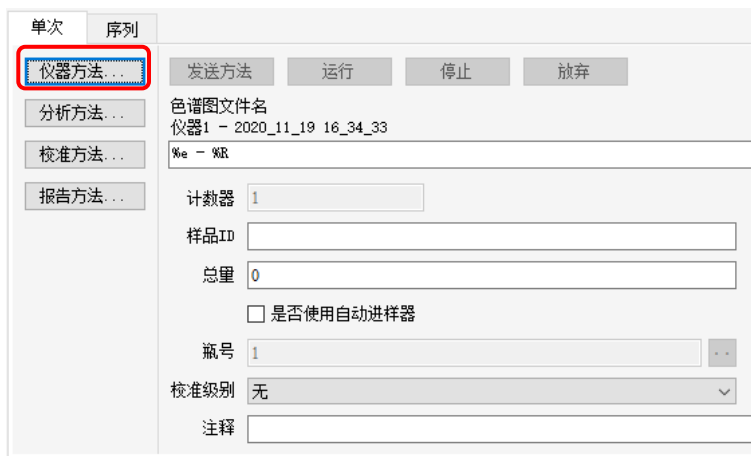
Figure 3-3 Instrument method setting interface of the Kromstation workstation
