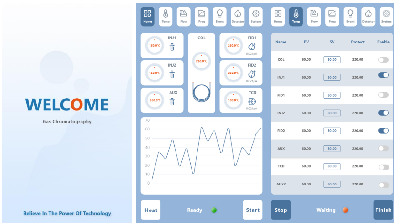
Fig 3-1 Viewing and setting the temperature control function
