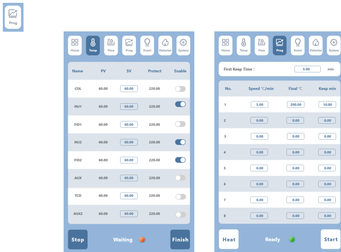
Fig 3-2 View and setting of program temperature rise
