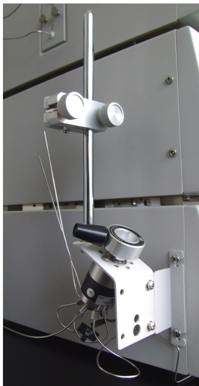
Fig.3: ZJ-1 valve bracket and manual injection valve
