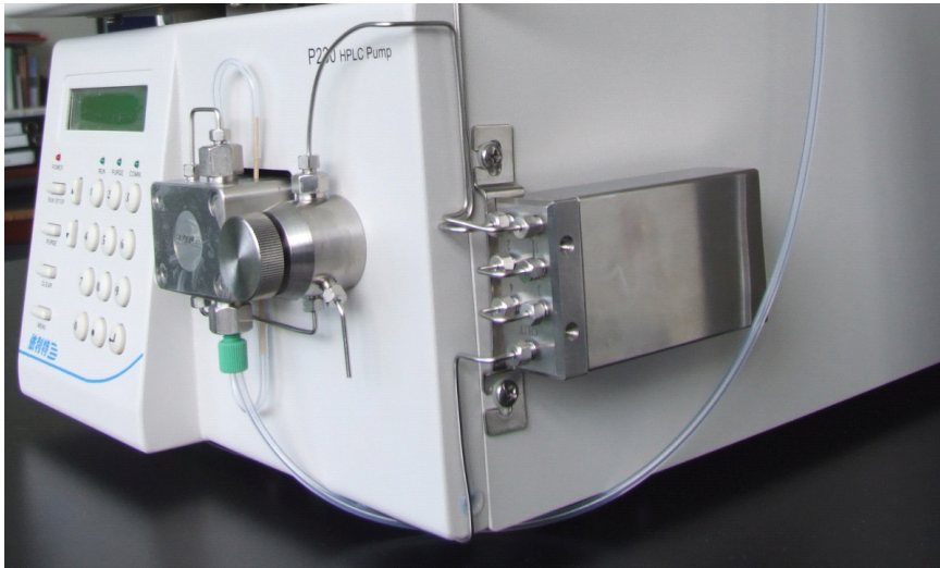
Fig.4: gradient mixer and pump A
